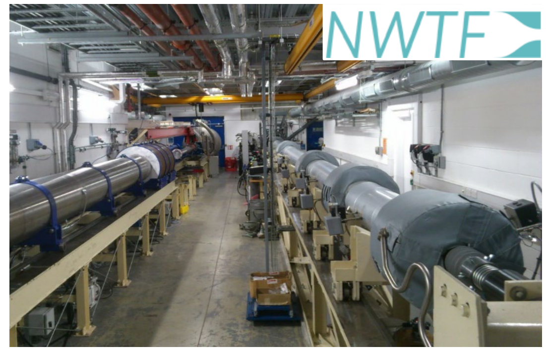
Oxford Hypersonic Wind Tunnels. T6 is on the left and the High Density Tunnel on the right .
